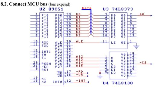
The CH372 has the common passive parallel interface, connects to various uPs $_{\circ}$ DSP and MCU directly. In common MCS-51 typical application circuit, CH372 can connects to system bus of MCU U2 through 8-bit passive parallel interfaces D7 $_{\circ}$ D0, -RD, -WR, -CS and A0.
